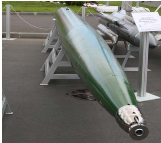
Figure 17. VA-111 Shkval Super-Cavitation Rocket-Propelled Torpedo From [57]
