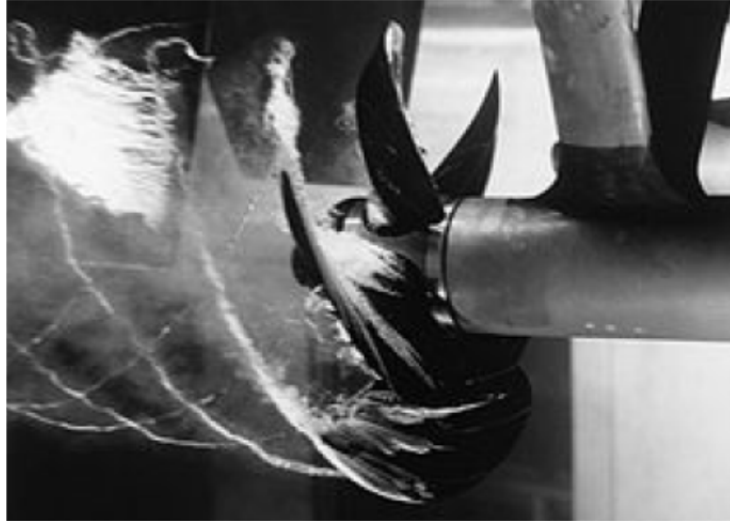
Figure 51. Cavitating Propeller Model in a Water Tunnel Experiment From [111]
