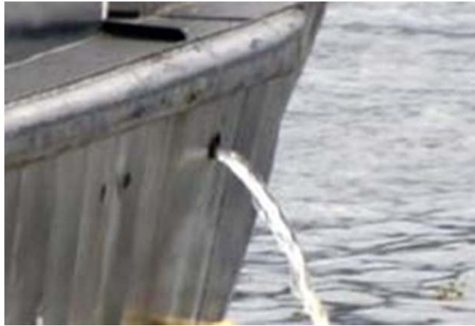
Figure 33. Bilge Pump Outlet of a Ship From [90]
