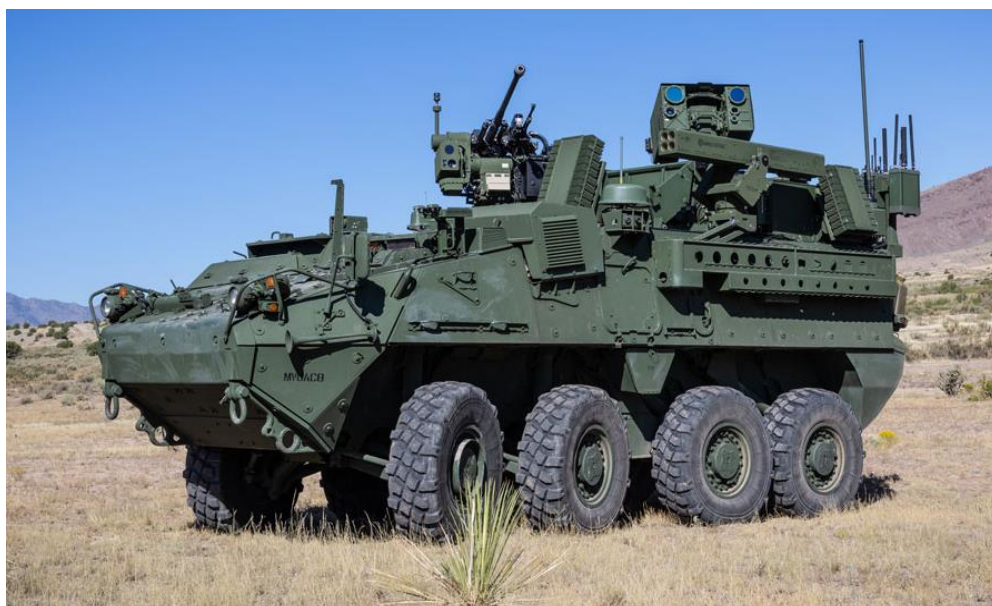
Figure 6. Leonardo DE C-UAS air-defense system on trials (Leonardo US Inc., 2024).
