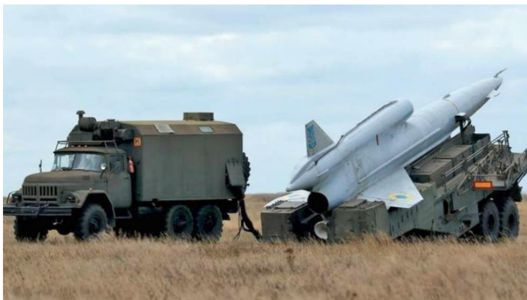
Figure 1. Tu-141 – a typical unmanned aerial vehicle from the end of the Cold War (Rogoway, 2022).
