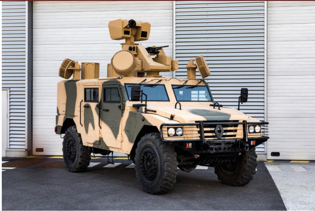
Figure 3. The HELMA-P laser system (Michau & Védrenne, 2024).
