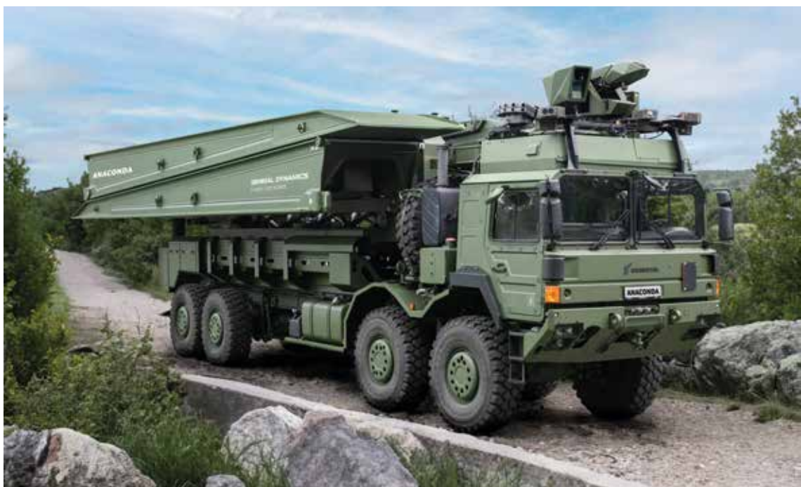
▲ Pictured: Anaconda, based on the earlier Beaver system. Re-engineering is one way to upgrade and increase bridging MLCs. [GDELS]
