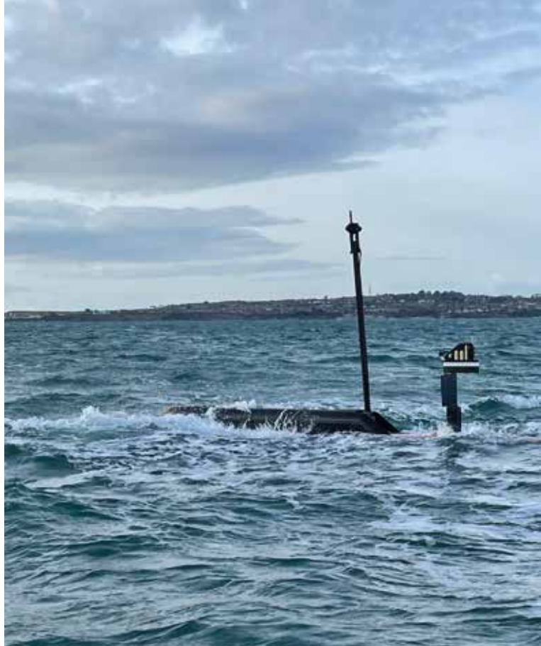
▲ The Herne XLAUV demonstrator pictured on the surface with its ISR mast extended. [Richard Scott/NAVYPIX]
